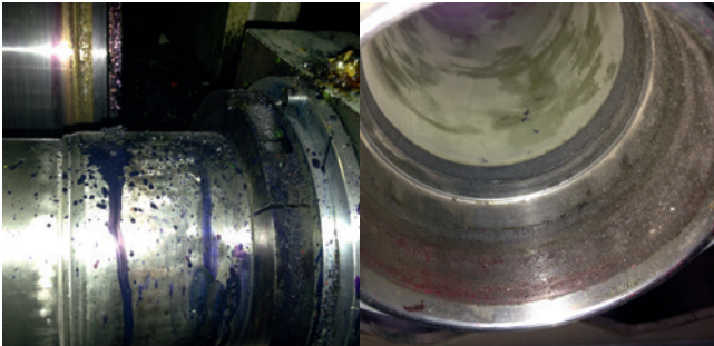
Dirt and surface damages on the carbon fiber adapter affect immediately the process safety of the flexo printing.
