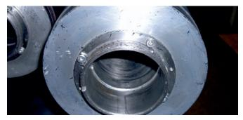
Dirt and surface damages on adapters effect directly the process safety in the flexo print.
