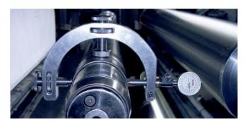
By using high precision measuring tools and calculating programs, SWT Services rates the complete system, consisting of clamping cylinder and adapter, right at the machine.
