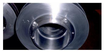
Cleaned, ground and measured all adapters can be easily fitted and precision clamped on to the clamping cylinder.
