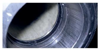
Grooves, rills, marks on the clamping surface of the cylinder and adapter can be one reason, that the adapter cannot be fitted smoothly onto the cylinder.
