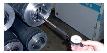
After cleaning, checking and repair all clamping areas get measured to ensure proper function.
